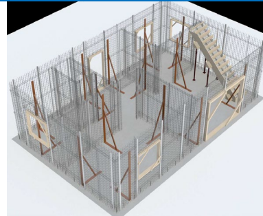
ASSEMBLED PANELS AND BEAMS
